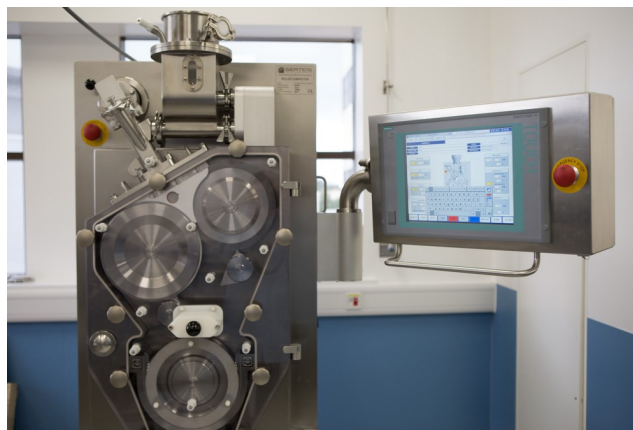
Instruments (fluid bed dryer and roller compactor ) used in Macclesfield for tablet making.
