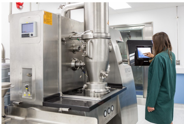
Instruments (fluid bed dryer and roller compactor ) used in Macclesfield for tablet making.
